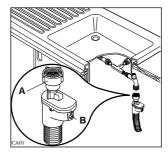
The problem is signalled by a red indicator which appears in window (B). If this happens, close the water tap and have the hose replaced.
